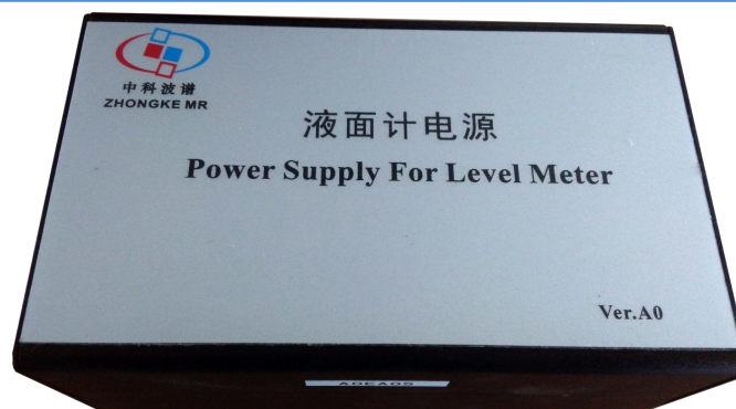
Fig. 2 Level meter power supply
