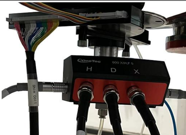
Figure 15. Connection of RF cables
