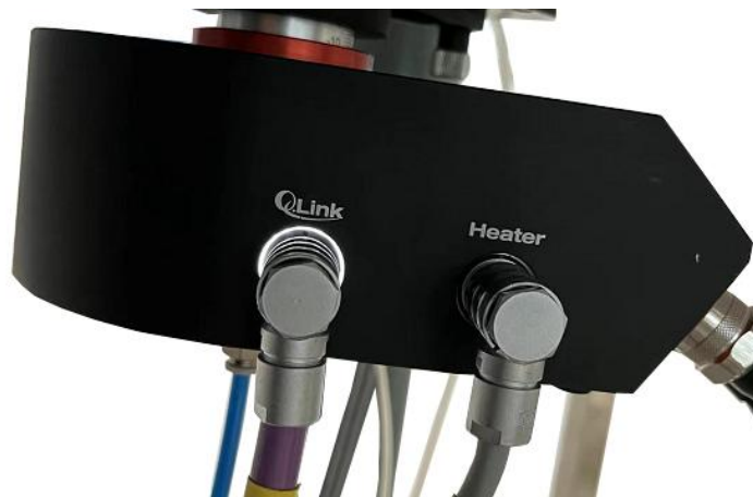
Figure 18. Connect Q.Link and Heater cable
