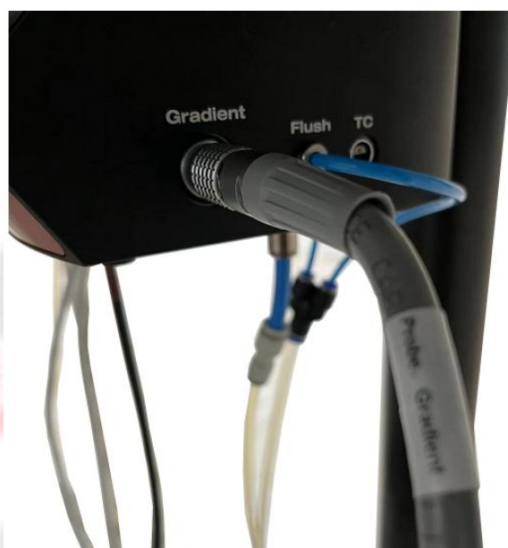
Figure 16. Connect the Gradient cable and the flush gas(4mm)
