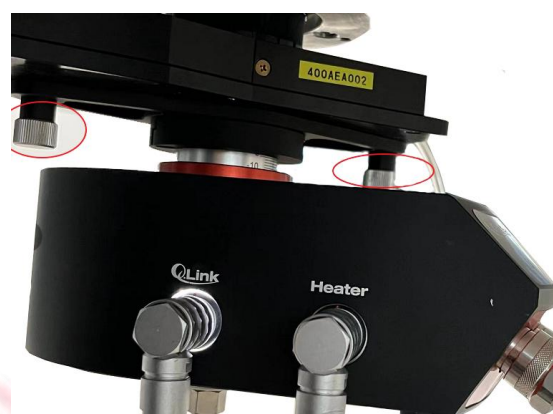
Figure 13. Insert the probe and tighten the two hand screws.
