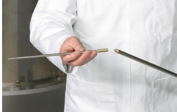
Figure 6 Fit syphon extension to dewar leg
