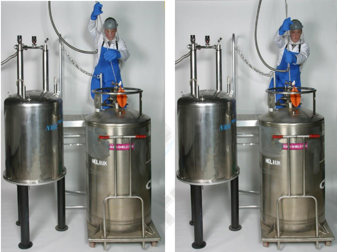
Figure 12 Inserting syphon leg into storage dewar
