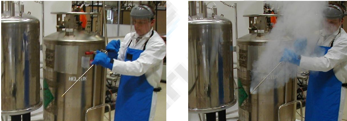
Figure 14 Pre-cooling the syphon
