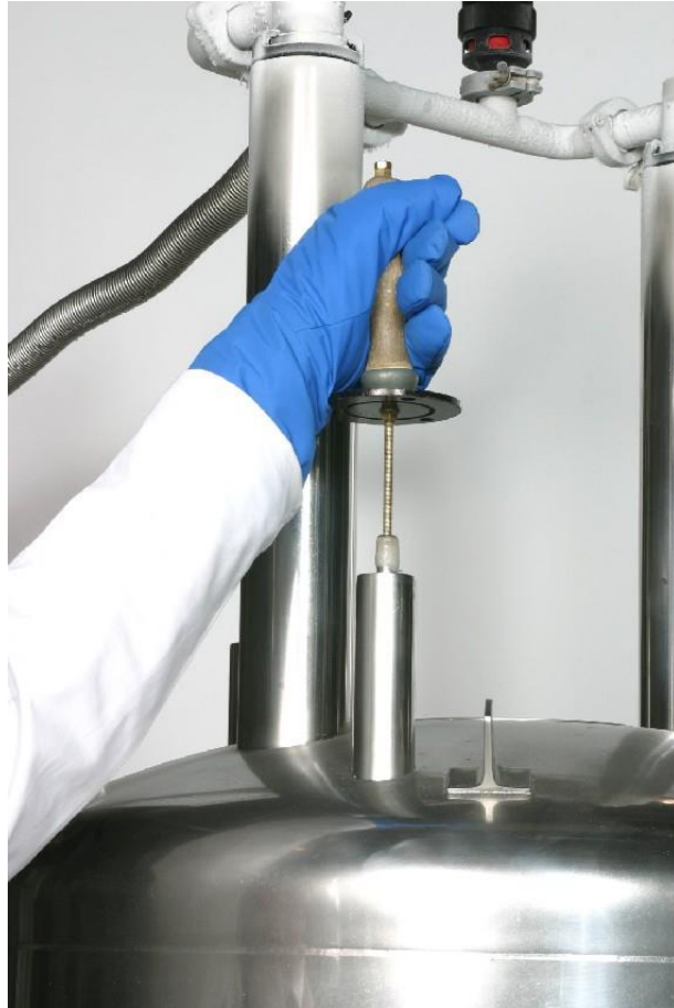
Figure 21 Use of a simple tool to check for ice blockage in nitrogen port
