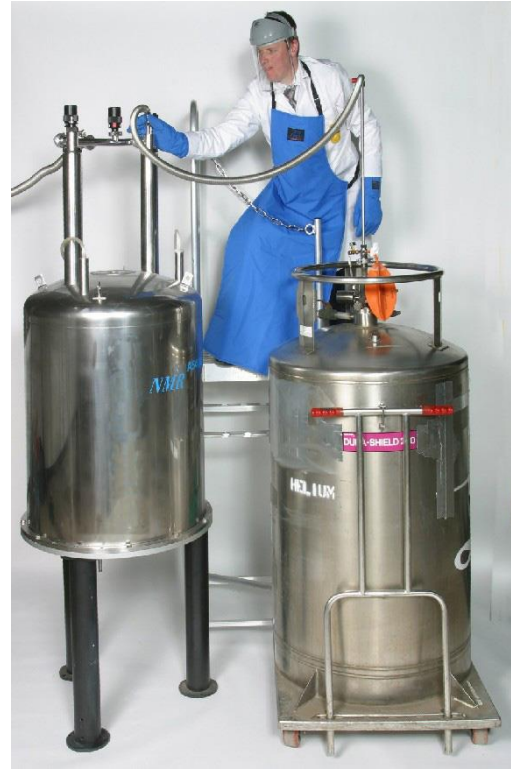
Figure 16 Inserting syphon leg into cryostat and making a gas tight seal
