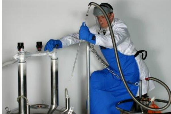
Figure 20 Syphon leg just after removal from cryostat
