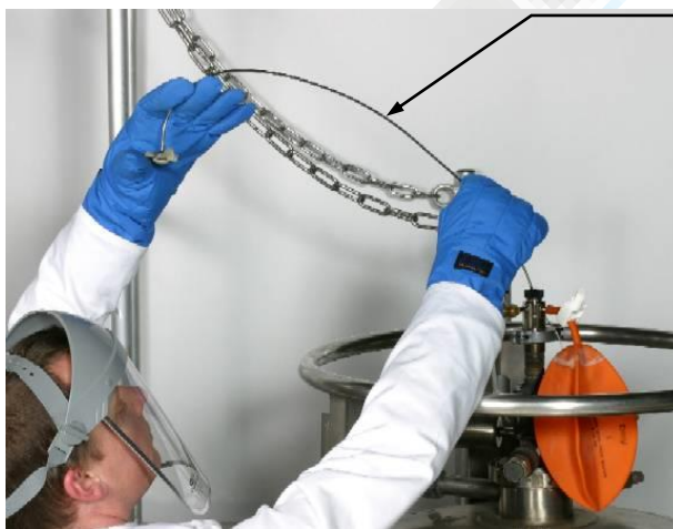
Figure 3 Using a dipstick to measure helium level
