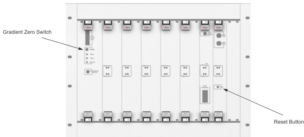
Fig. 22 Location Diagram of Reset Switch of Magnetic Field Regulation System
