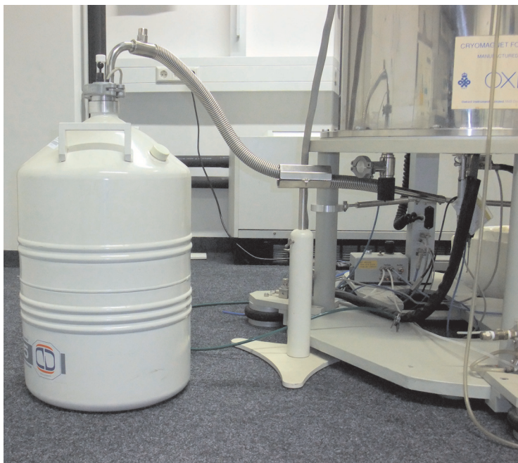
Fig. 8.5-4 Typical set up for low-temperature NMR measurements
