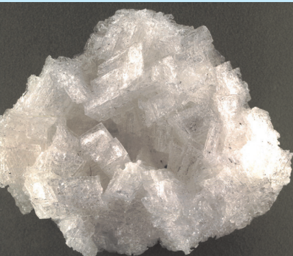
Fig. 4.2-2 Nitratine ( \text{NaNO}_3 ) – a nitrogen – containing mineral which can be found in the Atacama desert, Chile. Photograph as a courtesy of Dr. H.-J. Höbler, Mineralogical Collection University of Leipzig.
