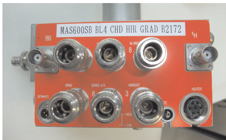
Fig. 7.2-2 Base of HR-MAS probe (Bruker) with r.f. and air connectors
