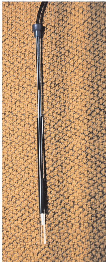
Fig 8.5-7 A Pt-100 resistor in an NMR tube filled with silicon oil for measuring temperature in situ
