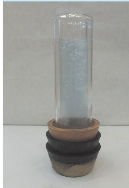
Fig. 4.3-1 Liquid oxygen in a transparent dewar with its typical pale blue color
