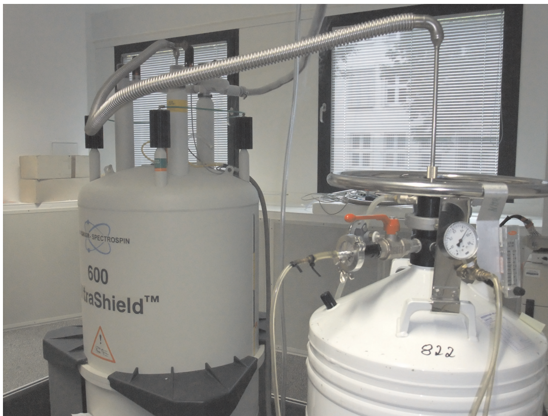
Fig. 8.0-1 Helium refill on a 600 MHz instrument
