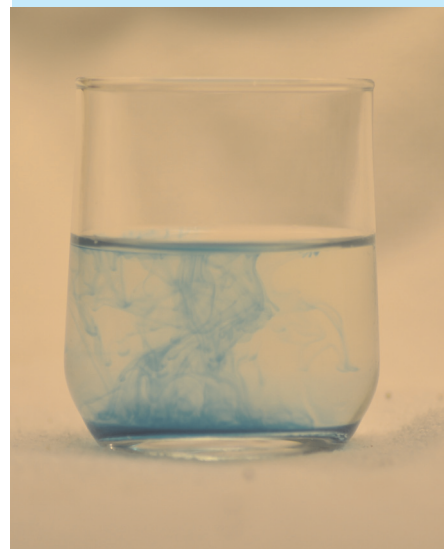
Fig. 5.4-1 A drop of ink diffusing in water
