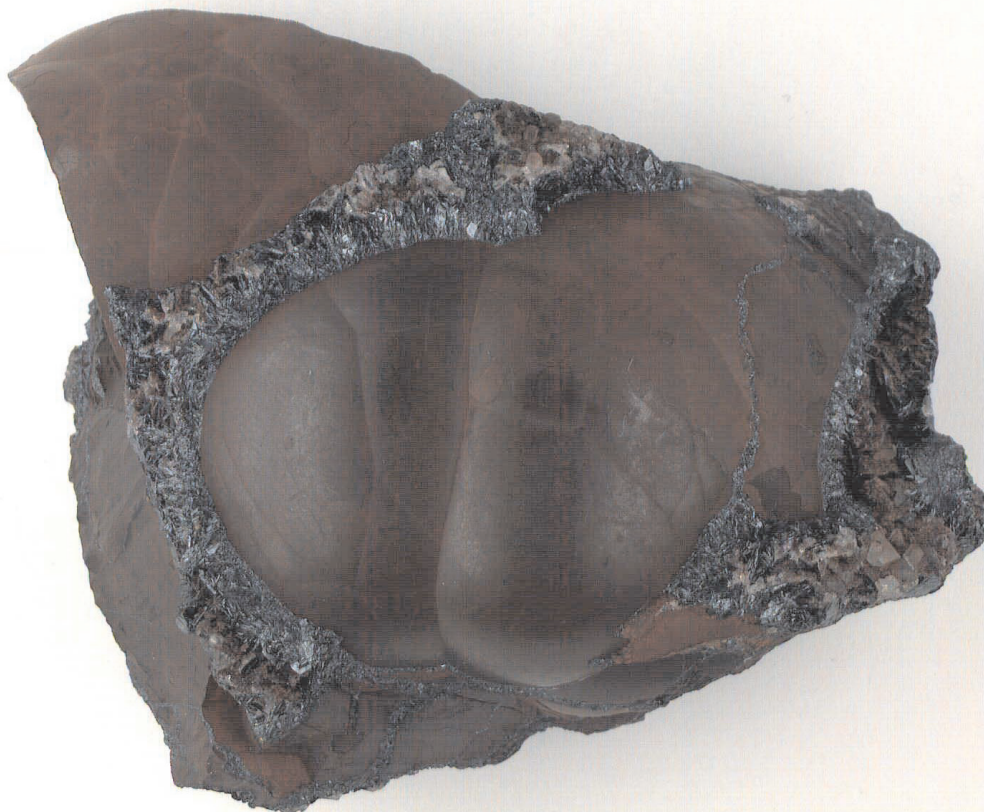
Fig. 4.6-4 Hematite (blood ore) \text{Fe}_2\text{O}_3 , from Cumbria (UK), photograph by courtesy of Dr. H.-J. Höbner, Mineralogical and Petrographical collection, University of Leipzig.
